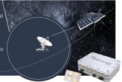
XLink is an advanced transceiver system (Software Defined Radio – SDR) for X- and S-Band communication links of small satellites with a flight grade tested COTS design. The mechanical dimensions fit into CubeSats as well as larger satellites. Radio interfaces and protocols are compatible to standard CCSDS and DVB-S2 specifications. Gigabit Ethernet is provided as on-board control and high-speed data interface
